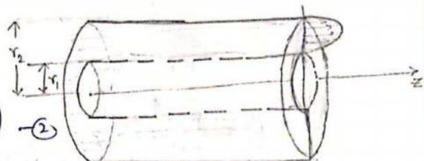
$$\frac{1}{4\mu} \frac{dp}{dz} (r_1^2 + A \log r_1 + B) = 0 \quad \dots \quad 3(i)$$
