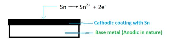
The best example of cathodic metal coating is Tinning. Tinning is a process in which coating of base metal (to be protected) takes place by dipping the base metal (anodic in nature) into the molten Tin (cathodic in nature).
