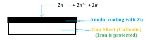
The best example of anodic metal coating is Galvanization. Galvanization is a process in which coating of base metal (to be protected) takes place by dipping the base metal (cathodic in nature) into the molten zinc (anodic in nature).
