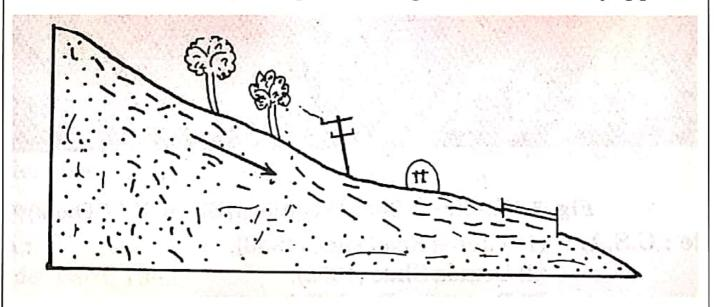
If water saturated materials are involved soil creep is called solifluxion and when it it's a wet mud without vegetation mud flow. Mudflows are common in areas effected by wild forest fires and on slopes of volcanic cones.
