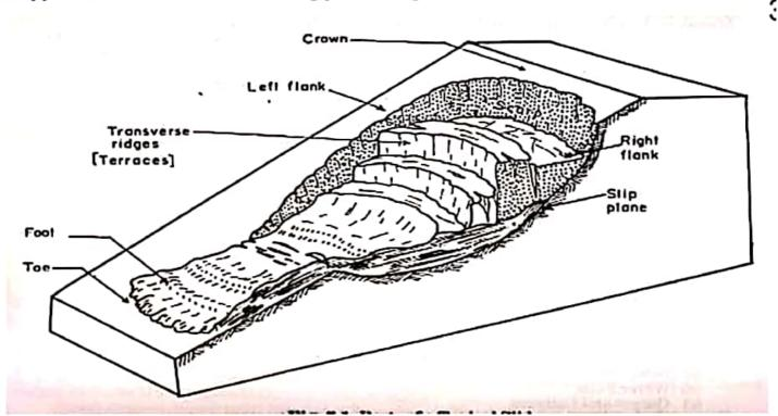
**CROWN**: - The upper portion still in place from which solid rock and soil materials are torn away from the rest of the slope.
