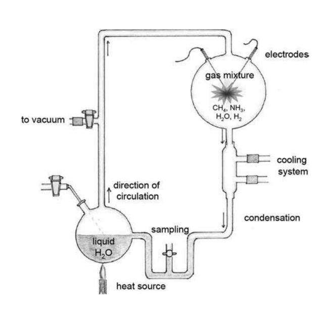
*Miller–Urey experiment set-up, which simulates in the laboratory the coupled chemistry between the primitive Earth atmosphere (upper right bulb) and warm oceans (lower left bulb). In the first version, an atmosphere made of CH<sub>4</sub>, NH<sub>3</sub>, H<sub>2</sub>O, and H<sub>2</sub> was considered. A spark discharge simulated storm lightning*
