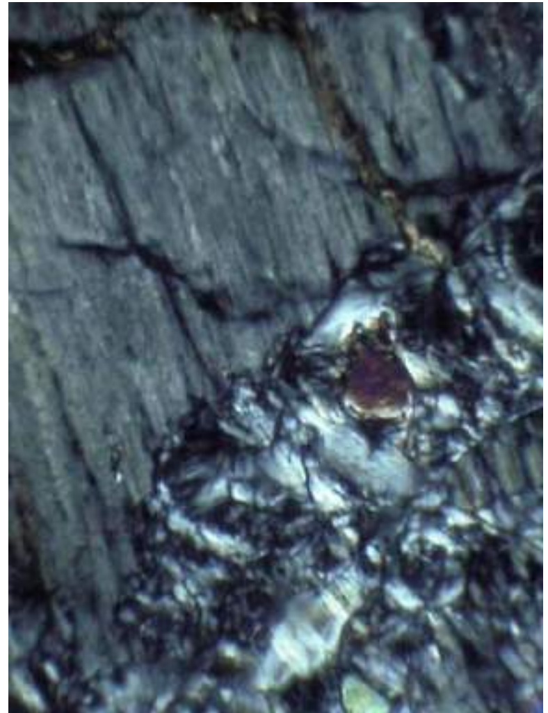
Figure. b. Serpentine pseudomorphs orthopyroxene to form bastite in the upper portion of photograph, giving way to mesh olivine below. Field of view ca. 0.1 mm.
