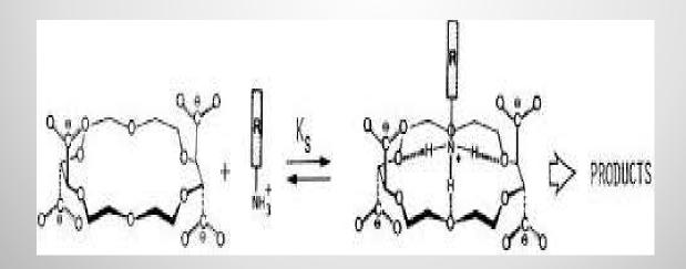
Ester cleavage process most frequentaly found in Enzyme model studies. Macrocyclic polyether with side chain bearing bearing thiol groups cleave activated esters with rate enhancement and chiral discrimination
