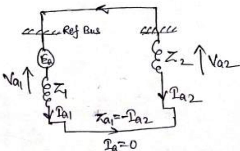
Eqn. (14) shows that the three sequence N/H's are connected such that the zero sequence N/H is absent and only the positive and negative seq. N/H's are connected in series-opposition to simulate the LL fault as shown in above fig.
