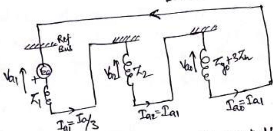
Eqn. ⑦ derived as above implies that the three seq. networks are connected in series to simulate a L-G fault. further the following relations satisfied under the fault conditions —
