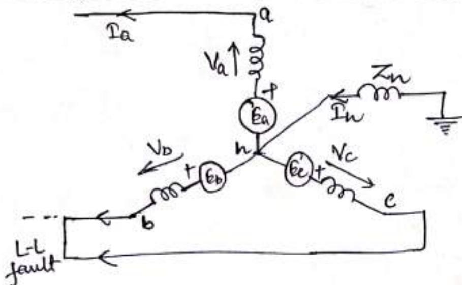
Consider a line-to-line (L-L) fault between phase 'b' and 'c' as shown in fig., at the terminals of a conventional (unloaded) generator, whose neutral is grounded through a reactance. Consider now the conditions under fault as under —
