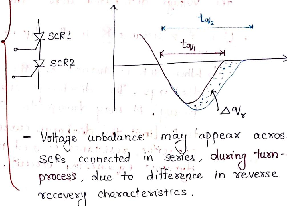
If both the SCRs have same reverse recovery characteristics, then they turn off simultaneously. So, they will share the total voltage equally.
