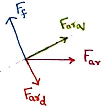
Stabilizing action of the air-gap reaction force due to residual magnetism.
