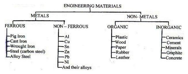
**METALS:** Metals are generally solids and have good heat electrical conductivity, good malleability and ductility, high melting point and high strength. These can be further classified as:
