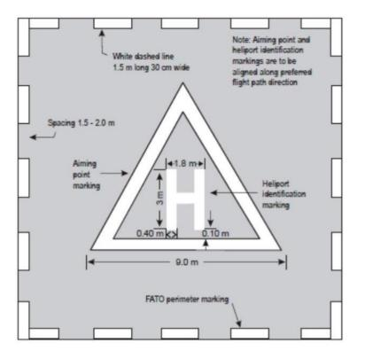
The heliport must be identified by the letter H in white, placed in the interior of the FATO, at the centre or near the centre of this and placed in such a way that the "horizontal" bar of this letter is perpendicular to the preferred direction of approach. This H is 1.80 metres wide and 3.00 metres in height and is constructed with the aid of 0.40 metre width bars.
