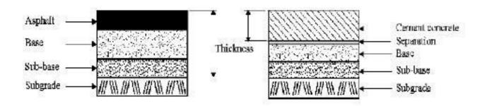
Flexible pavements typically consist of bituminous "surface course," a "base course," and a subbase course." These courses or layers are carefully placed and compacted on a prepared subgrade in an embankment or excavation.
