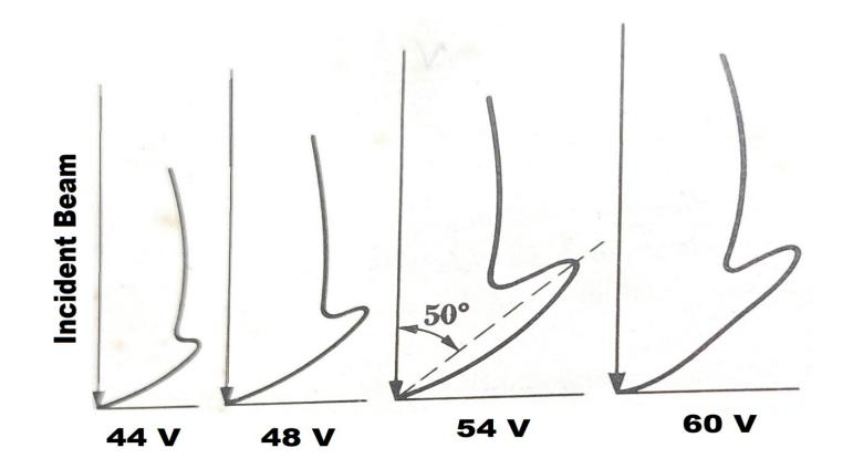
The method of plotting is such that the intensity at an angle is proportional to the distance of the curve at that angle from the point of scattering two questions
