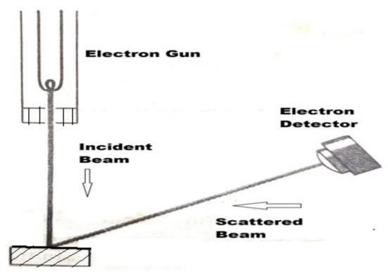
According to the classical physics the scattered electrons should emerge in all directions with only a moderate dependence of their intensity upon scattering angle and even less upon the energy of the primary electrons.
