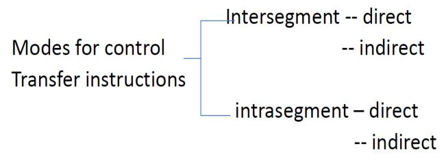
Fig 2.1 Addressing modes for control transfer instructions
