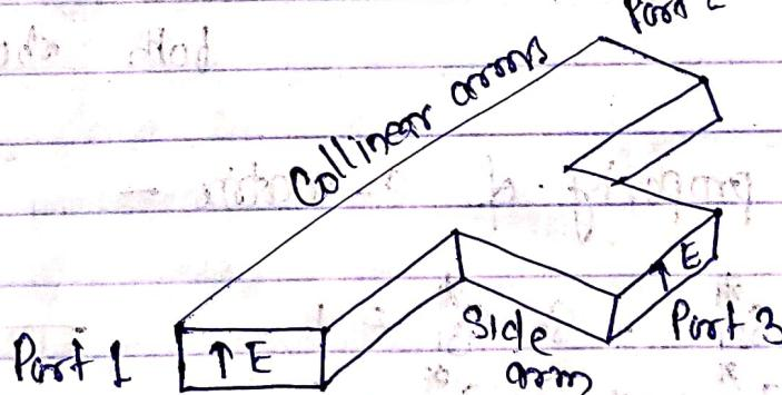
\* If two input waves are fed into port 1 and port 2 of the collinear arm, the output wave at port 3 will be in phase and additive.
