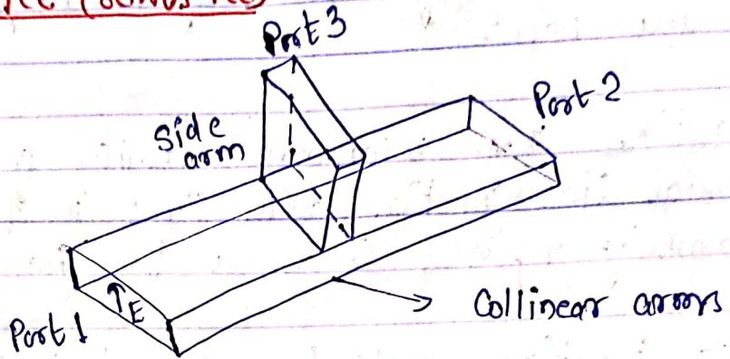
\* An E-plane tee is a waveguide tee in which the axis of its side arm is parallel to the E field of the main guide.
