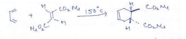
The stereochemistry of diene is also faithfully transmitted to the product. Diene adds to an acetylenic dienophile to give the cis product.
