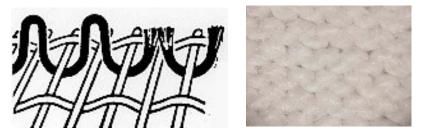
Pile refers more to the third thread used to make a thick fabric. The third thread is looped up and down through a plain weave.
