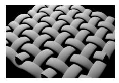
Plain weave patterns have each thread going over then under (then over then under then over then under...) each crossing thread. A "tight" pattern means that parallel threads are tight to each other (no space between them).
