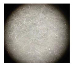
Fibers in non-woven fabrics are randomly placed on each other and the fabric is then pressed. There is no discernable pattern.
