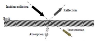
The incident electromagnetic energy may interact with the earth surface features in three possible ways: Reflection, Absorption and Transmission.
