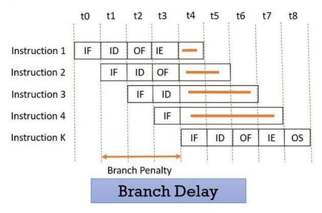
Prefetching the target branch address will reduce the branch delay. Like if the target branch is identified at the decode stage then the branch delay will reduce to 1 clock cycle.
