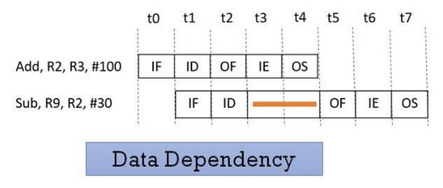
In the figure above, you can see that result of the **Add** instruction is stored in the register **R2** and we know that the final result is stored at the end of the execution of the instruction which will happen at the clock cycle **t4**.
