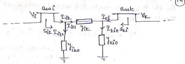
1- representation of a line and transformers connected blw two buses
